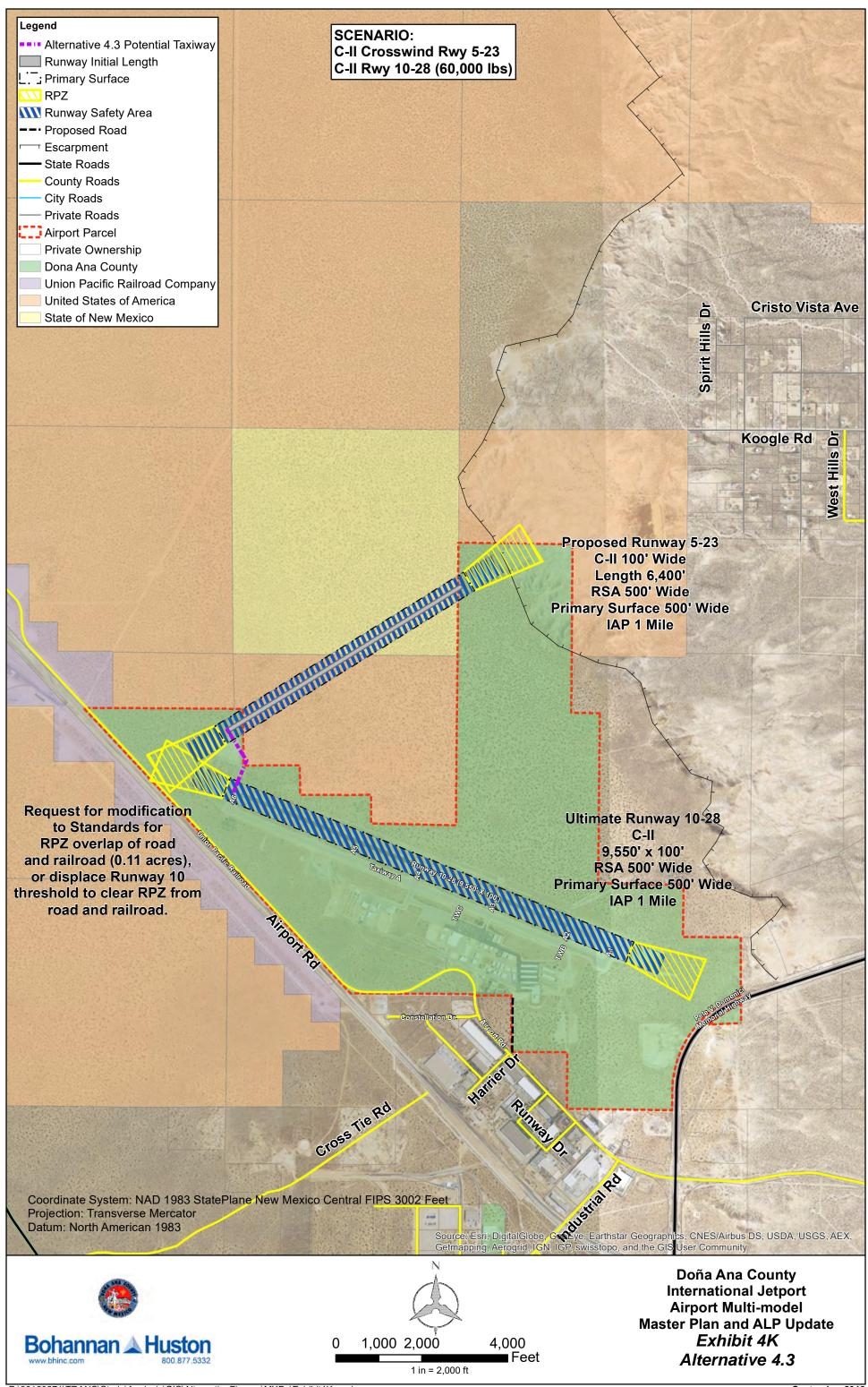
alignments were included in the wind analyses to determine which runway alignment provides the best wind coverage. The green bar on the exhibit represents the wind coverage for each individual runway and the blue bar represents the total combined wind coverage of Runway 10-28 and each proposed crosswind alignment.
